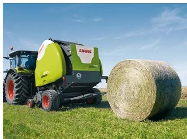
As before, there are four models and two bale sizes in the VARIANT 400 range. With the VARIANT 460RF and 465RC, the bale size is variable from 0.90m up to 1.55m, while bales up to 1.8m can be created using the VARIANT 480RF and 485RC.
